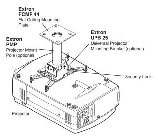
Figure 4. Typical Application of FCMP 44
